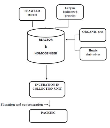
Though the basic process for manufacturing of Bio Products, as illustrated above, remains same, various products have some additional processes. Also, majority of products follow repeat processes from Reactor to Incubation and then to filtration and concentration processes.
